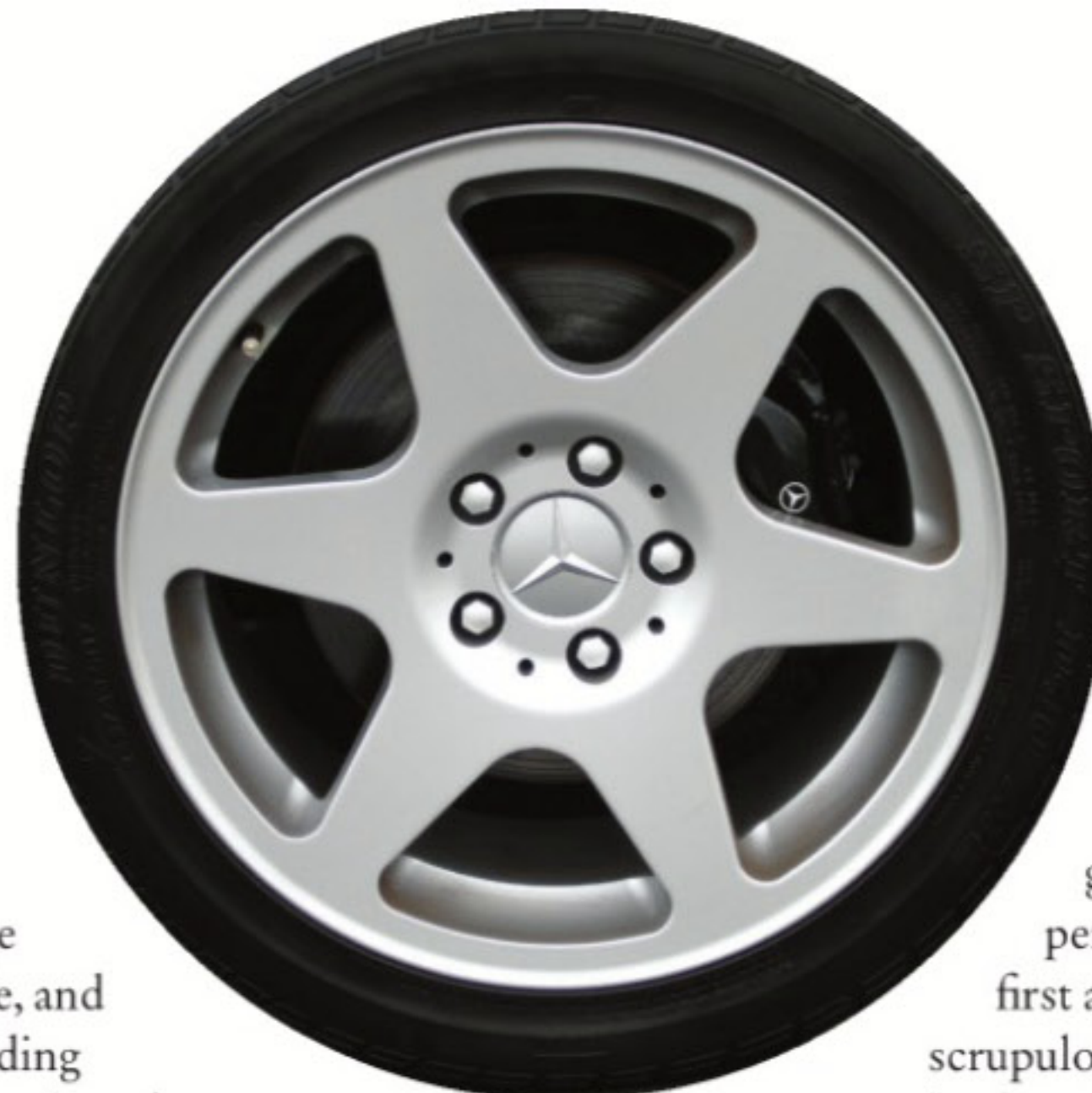
▲ 245/50ZR17 rubber – widest and lowest profile of any 190E.
